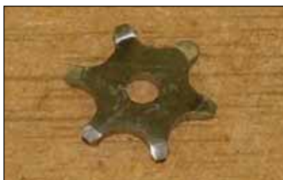
Here's a close-up of the finished spur (six-point) gear, which attaches to the wiper motor.
