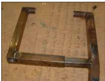
This is the assembly of the two sliding pieces that clamp onto the nosegear tow pins. There is a tension spring inside that holds the two halves onto the nosegear.
