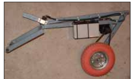
The tow hook can fold for storage in the baggage compartment. Folded length is 31 inches; it weighs 19 pounds with a battery.
