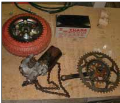
These are the main components: (1) the bike gear attached to the wheel, (2) the battery the author found at the junkyard, (3) the spur gear attached to the wiper motor, and (4) the bicycle gears from the dump.
