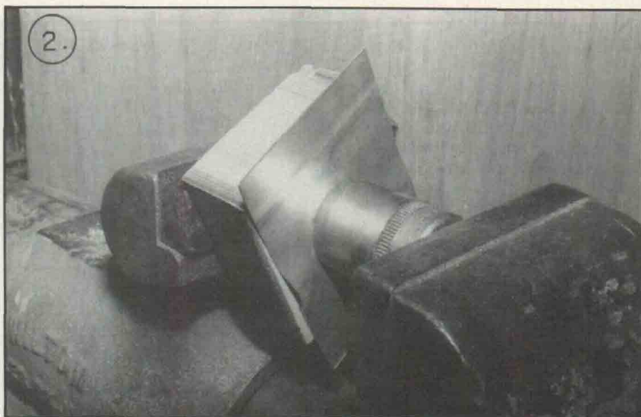
The first step in making a firewall shield is to take a piece of stainless, a soft pine block, a large socket, and insert this assembly in a large vise. Then, tighten the vise hard.
