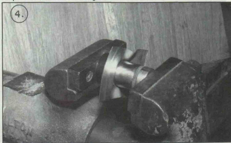
This view shows the third step. The socket, the stainless, and the large diameter tubing piece are assembled in the vise again. This time the squeezing will deepen the initial impression in the stainless piece.
