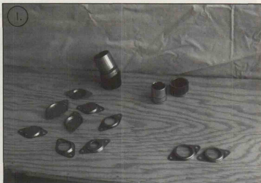
Here is all you need in the way of tools. A socket and a short section of tubing. Two different sizes are shown. In the foreground are a number of firewall shields in various stages of completion. The two on the right are "store bought" samples.
