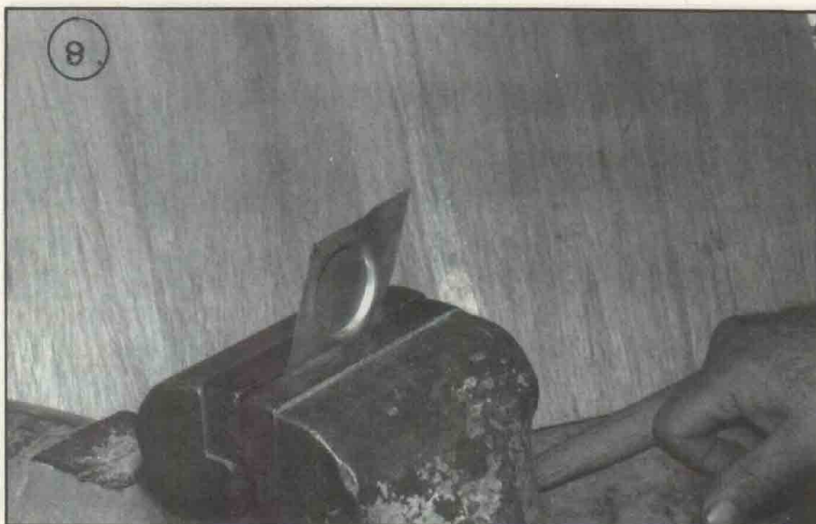
Continue straightening the edges. Notice now that a lot of excess metal has been cut away to make the straightening process a bit more effective.
