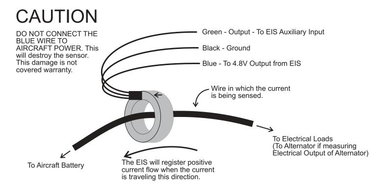
The Hall Effect current sensor measures the current flow in the wire that passes through it, without any electrical connection to this wire. Two locations for mounting the sensor are commonly used.
