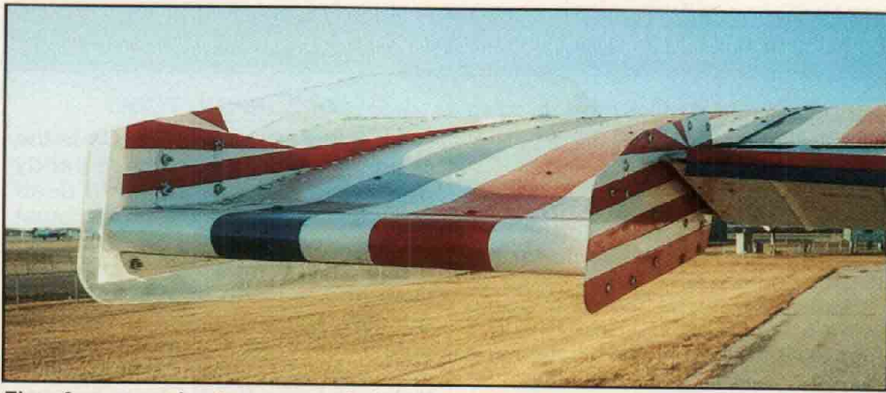
Flow fences and extreme rounded trailing edge of wingtip help the extreme low-speed effectiveness of this unique installation. The aileron "wedge" on the outboard end of the aileron is described in the article.
