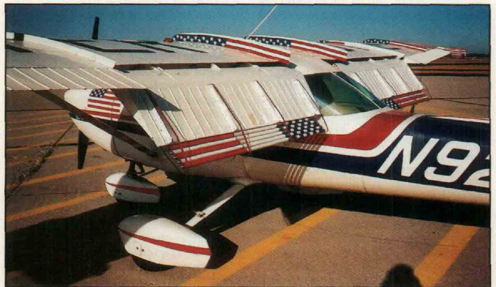
Full flap and "flaplet" deflection (plus flow fences on flaps) helps Don slow the 150 down to near zero airspeeds.
