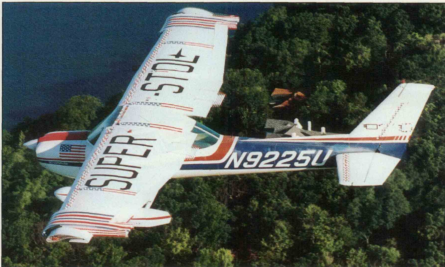
Called the Super STOL 150, the Cessna 150 reveals many of the modifications in this overhead photo. Note the extended "flaplets."
