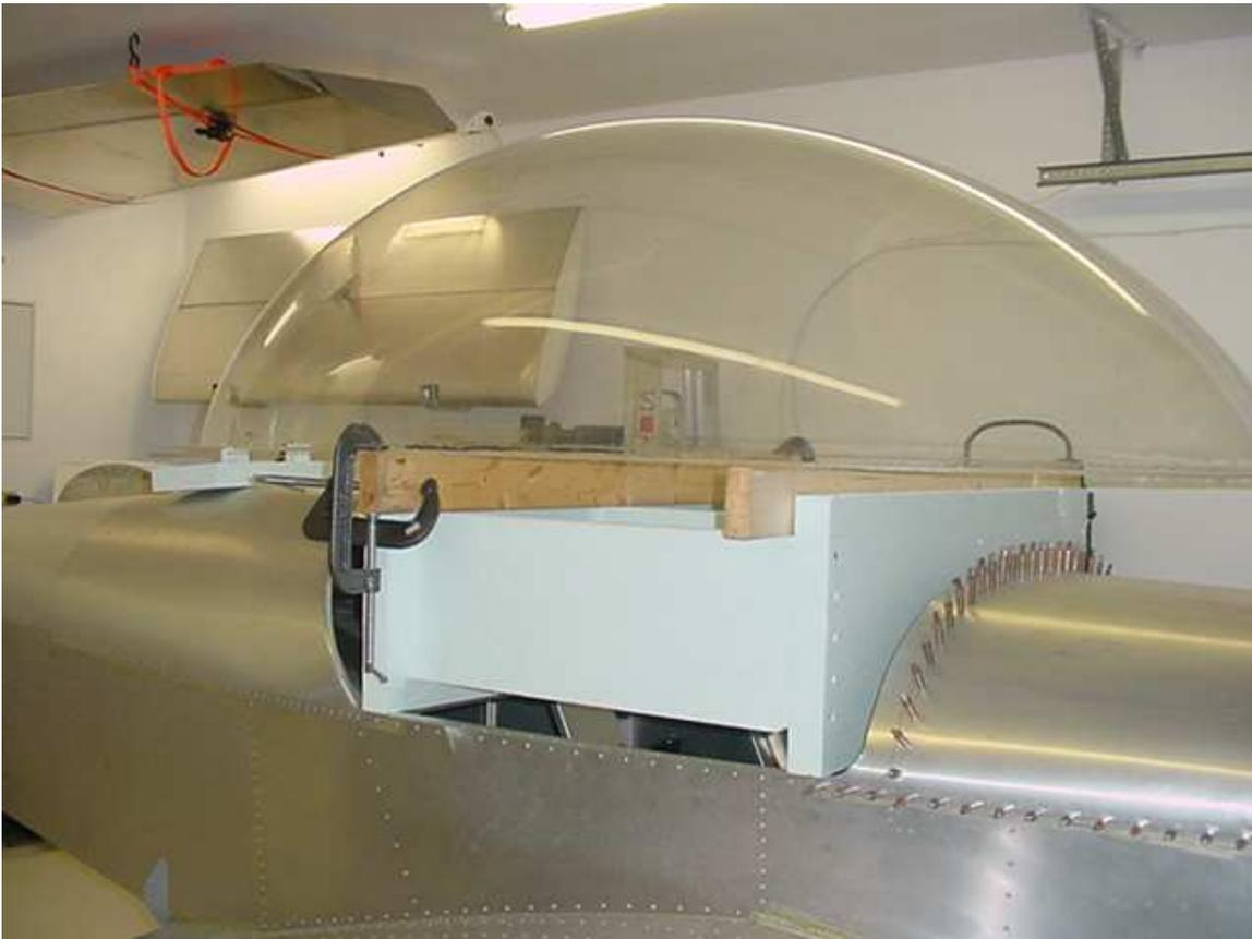
3. Place the canopy in position, over the fuselage
