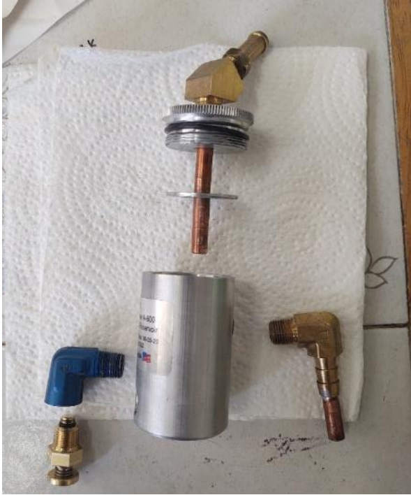
The can is small, and I used OO steel wool above the washer to filter out the oil spray.
