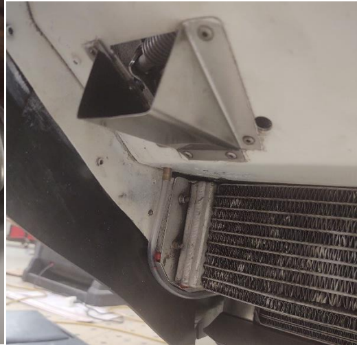
The drain is out of a drilled hole then will tuck under the rubber seal and exit the rear without any catch.
