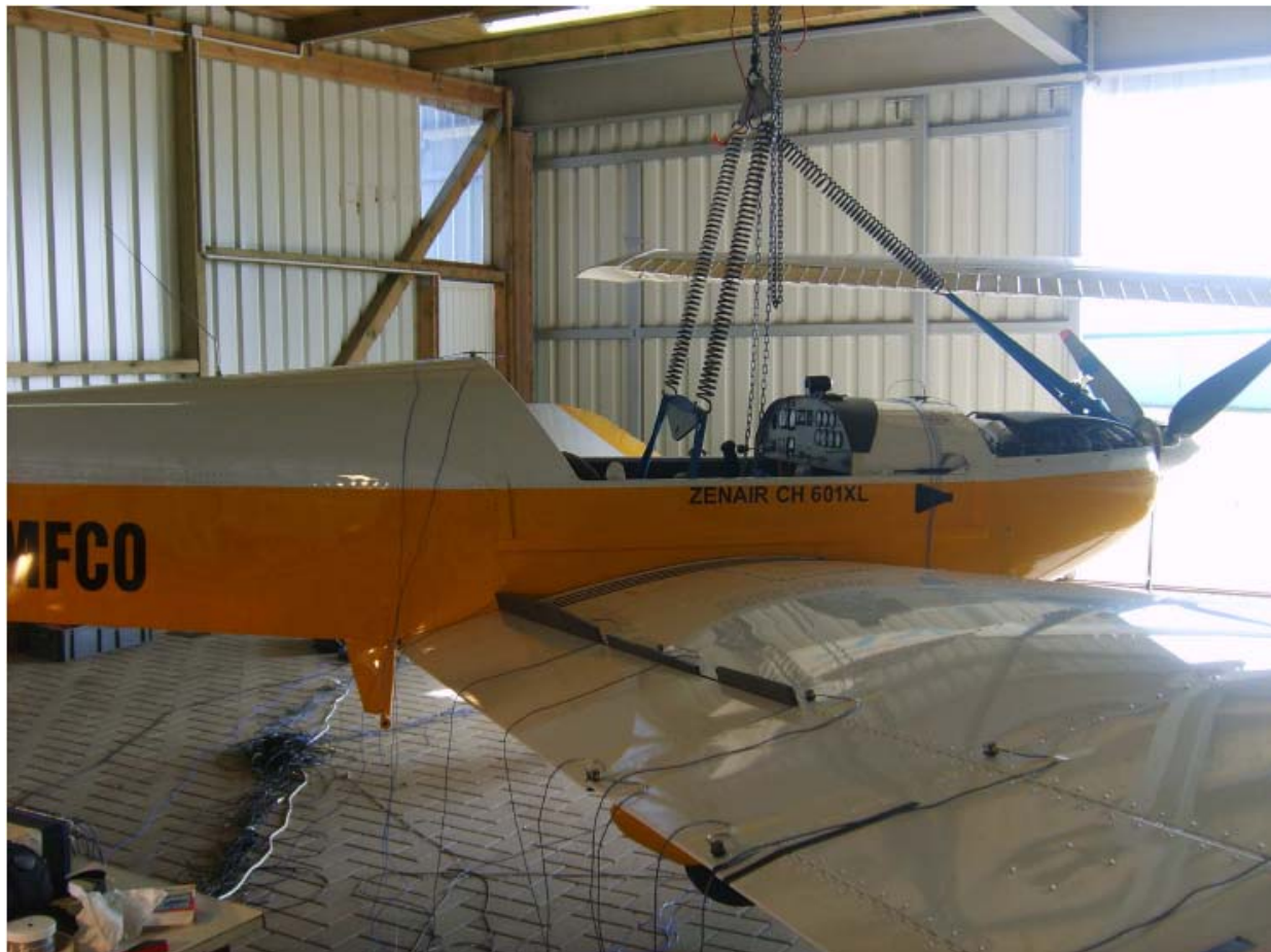
Figure 1: Ground Vibration Test CH601XL
