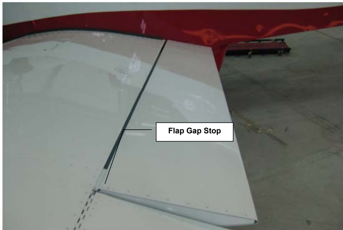
Figure 21: Flap gap stop, Part No. 6S3-1
