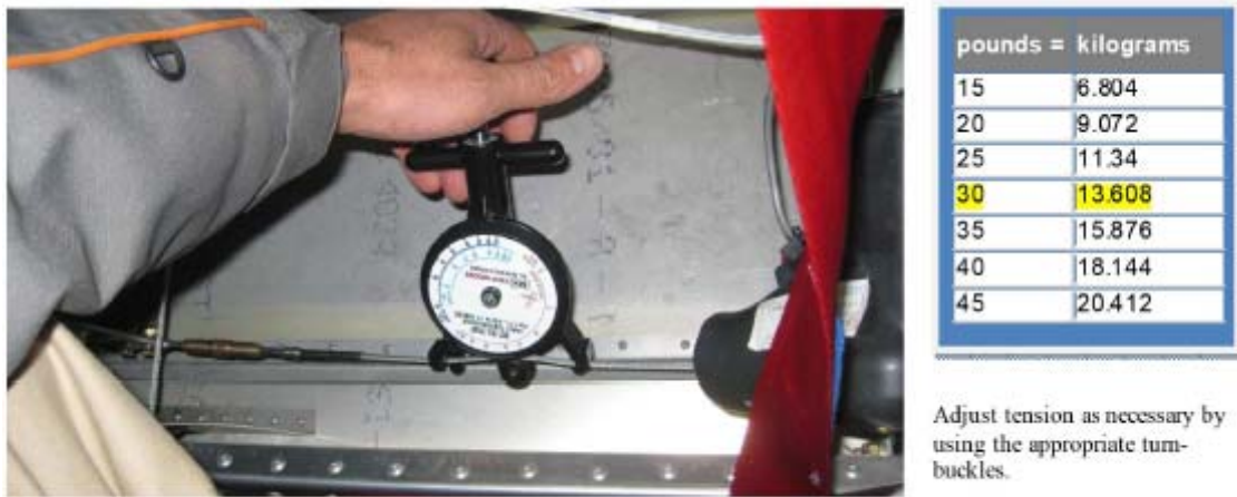
Figure 20: Adjusting control cable tension (see XLphotoguide.pdf)
