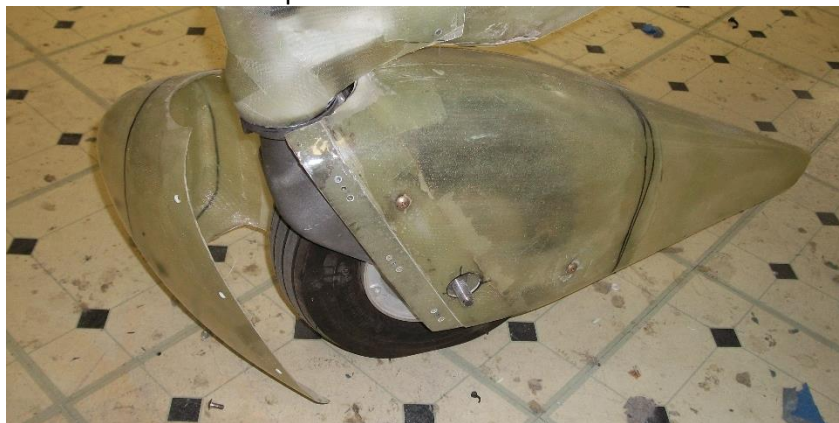
Nose pant during installation. The nose cone opens to allow access to the nose wheel tire valve.
