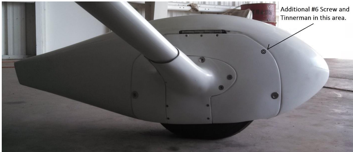
Original prototype and additional screw location to keep the inboard cover tight on the leading edge.
