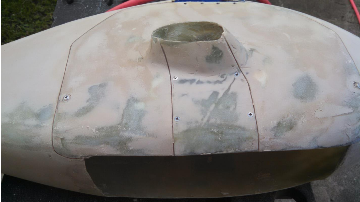
Above is the pant in fill and prep for final finishing.
