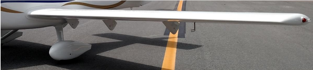
Wing cover speed kit finish installed.
