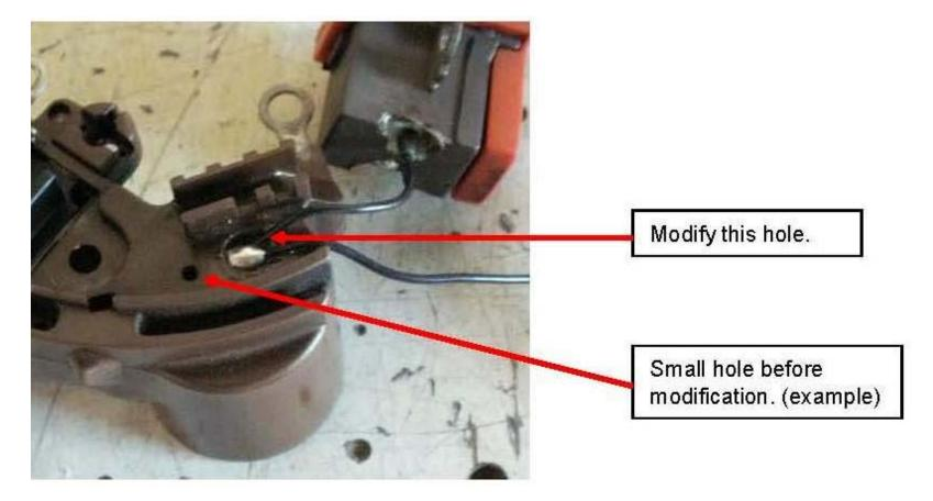
Mock-up assemble brush holder to regulator and route new brush feed lead to underside of regulator where modified previously. Solder new brush feed lead along with two more 22-ga leads (three total) to uncovered terminal.
