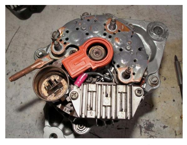
Hold rear cover over alternator and determine where to drill hole for crowbar lead pass-through:
