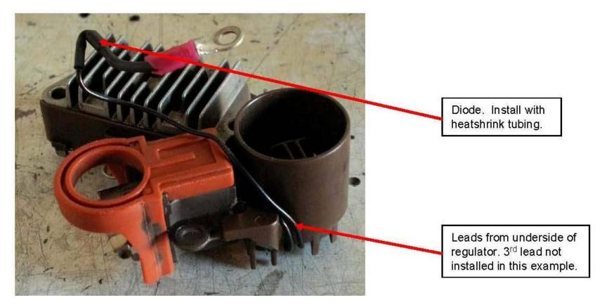
Route all three leads upward and reassemble regulator and brush holder into alternator. Solder one of the leads to the cathode of a 1A diode. Solder a 2" length of wire to the anode of diode and heatshrink. Crimp #8 ring terminal to anode end of diode lead and attach to a regulator hold-down screw. This diode will prevent pulse from collapsing field coil from back-feeding into regulator if/when 5A field breaker is pulled for testing with engine running.
