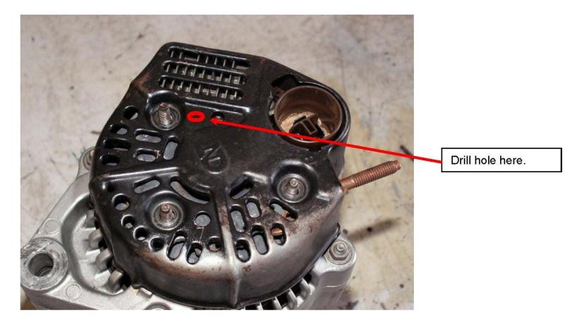
Drill hole and deburr and install rubber grommet.
