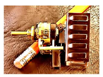
lights of the certificated aircraft you trained in, you turned a knob attached to an Ohmite Series-A wirewound rheostat. Somewhere behind the Royalite was a smoking hunk of ceramic wound with toaster wire. A finger holding a chiclet of graphite picked off the desired voltage. The whole thing weighed easily as much as a cheeseburger.
