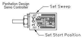
The function of these trimmers will be self-explanatory when the servo is operating. The 20k ohm trimmer will set the total sweep angle of the servo, the 5k-ohm trimmer will set the bottom-end start position. This change will make it easier to use the EGPNMSC in a variety of applications.
