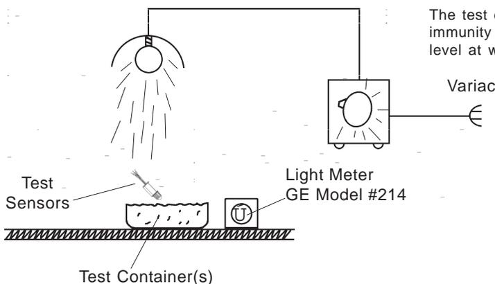
The test depicted below was performed to determine the sensor immunity level to ambient light. The recorded ambient is the maximum level at which the sensor performs/detects normally.
