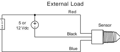
Note: May sink up to 40mA max. Use diode suppression for inductive loads.
