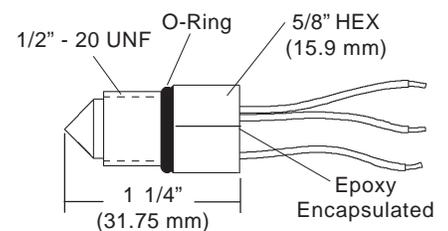
Electrical Termination: Lead Wires, 22 AWG, Polyester Jacketed, 6" to 6 1/2" Extended
