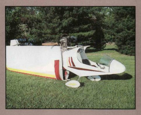
the spar. The 1.7 oz. Stits dacron fabric is glued to the rib tubes plus special pop riveting for a most secure bolt 'belt and suspenders' attachment. Two coats of Stits Polybrush and one coat of color finishes out the fabric.
