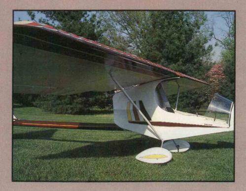
to the pilot and only slight airframe damage. It was an easy fix to stabilize the drag strut under high compression loads, so if a pilot somehow busts the 4 Gs limit he should be reasonably safe if he is gentle. If not, the ballistic chute could still save his bacon.
