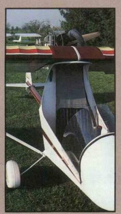
operated, with all cables carried inside the tail boom tube where they are protected against damage from disintegration of the prop. Some other ultralights in past years have been severely critized for their vulnerability in such a situation.
