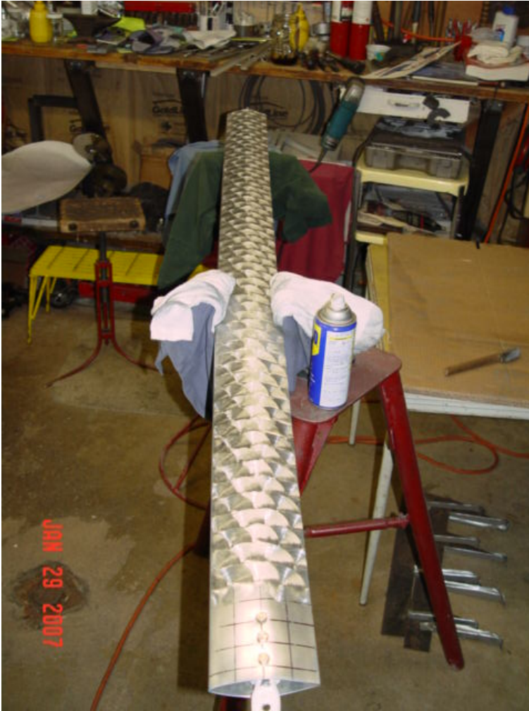
These things are a REAL BEAR to put on the curved surface Fish scales - Lift Struts 005.jpg (60.21 KiB) Viewed 6314 times
