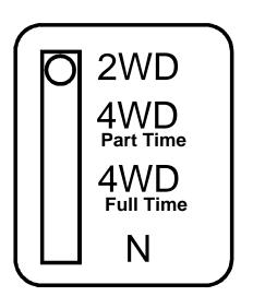
I can't resist throwing this in. My 2004 Jeep Grand Cherokee transfer case shifter: The top The 2WD is for two wheel drive—fixed two-wheel rear drive.
