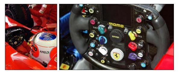
Here is an instrument panel built by Momo for a Ferrari grand prix racecar. Note that all the controls can be operated without letting go of the steering wheel. Note the digital display. Only Italians seem capable of designing with such flare! But Momo later toned this down considerably for the commercial market.
