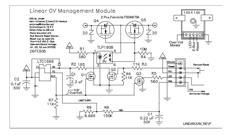
Description of Operation—The LTC1696 monitors the voltage Vbb through the voltage divider R8, R9. Inputs F1 and F2 when used together cause the LTC1696 to react faster to large dV/dt. The LTC1696 trigger is delayed 200 mS by Ct
