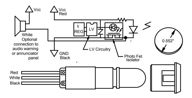
NOTE: For builders who want a steady, non-blinking LED, we have a steady LED version (please specify). The white wire can connect to either an audio warning or a light in the annunciator panel. If the white wire is not used, it can be left unconnected or clipped off short.
