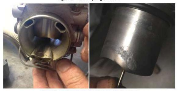
Figure 3 - Carburettor Contamination & Slide Wear
