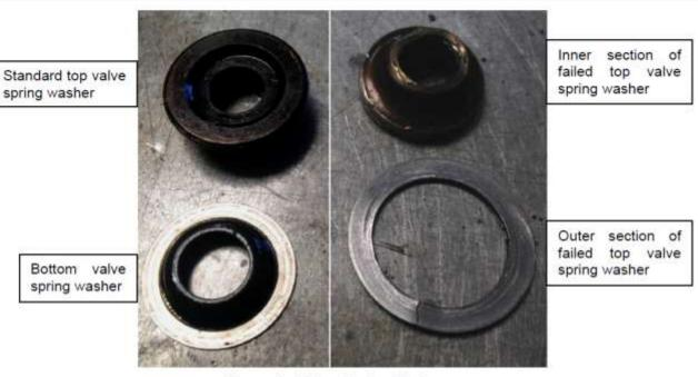
Figure 2 - Valve Spring Washers
