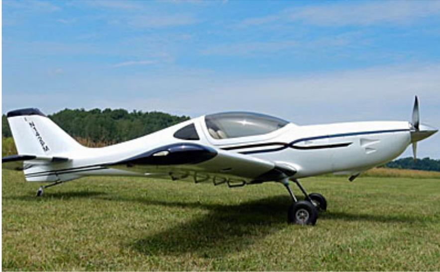
Lightning lives up to its name, running easily to the 120-knot maximum for LSA, especially when powered with a very muscular six-cylinder, 120 horsepower Jabiru 3300 powerplant. Every Lightning to date has been a tricycle gear airplane and, honestly, for most pilots, that is the right choice. However, like many aviators, I love the look of a tail dragger so when I stumbled across the one you see in the photos, I did a double take. *Whoa! That looks hot!*
