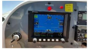
13,000 ft., 124 GS and a 30 mph cross wind! The OIT alarm was a loose wire on the temp sender. 5/29/2014
