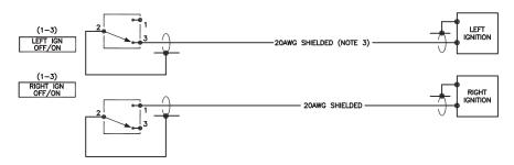
But the right mag is shown connecting its wire to terminal #1, not #3. So it seems the right mag is shown here with an ungrounded wire, so it would be ON. Yet the switch here is shown in the down position.
