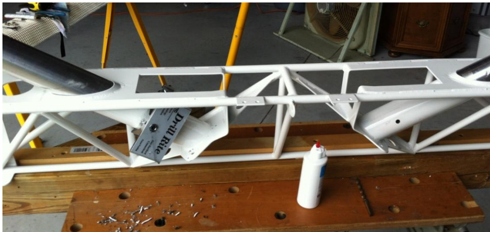
Figure 11: Drilling the gear holes (I used a Drill Rite guide).
