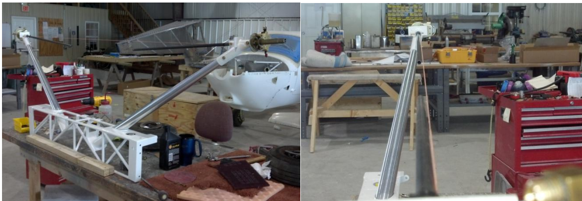
Figure 10: Setting the Toe (Factory pictures)
