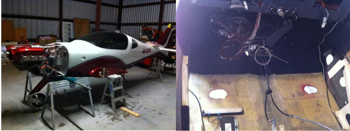
Figure 9: Plane on stands (left), Spar Box removed (right).
