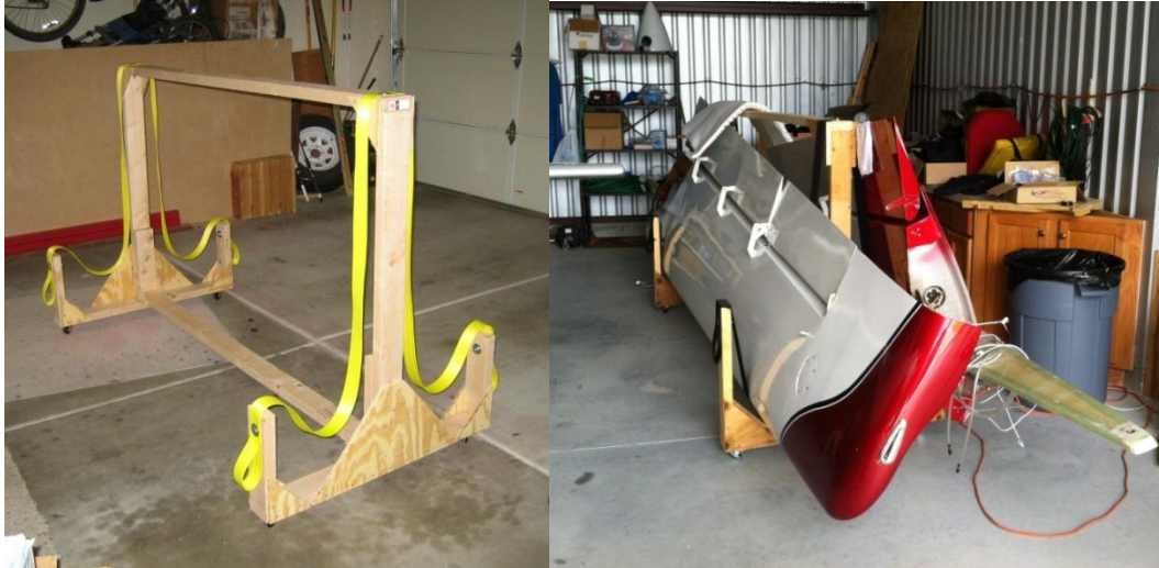
Figure 6: Wing Sling from the Web (left), Wings on my Wing Sling (right).
