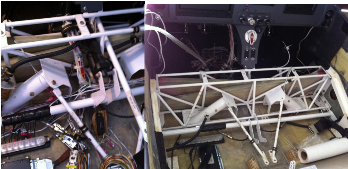
Figure 7: Before and after of wiring that runs through the spar box.
