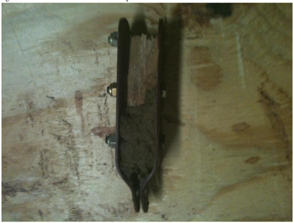
Here's a picture of the damaged left strut. You can see some deformation about a foot from the near end. Note, however, that the bolt holes are in great shape.
