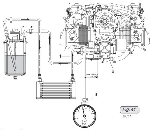
max. 0.3 bar (4.35 psi) below atmospheric pressure
