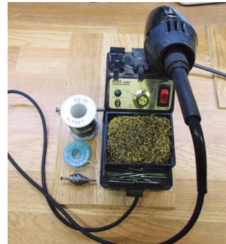
To the left of the soldering station (top to bottom) is a 16d “sinker” nail for large-diameter solder, one roll of 63/37 0.032-inch solder, Soder-Wick desoldering braid and 18 feet of 0.031-inch solder wound on a 12d “sinker” nail. The large knob on the panel controls temperature, and dry brass wool replaces the wet sponge that comes with the iron. Below the brass wool are extra soldering tips, which you probably won’t need if you use the brass wool.
