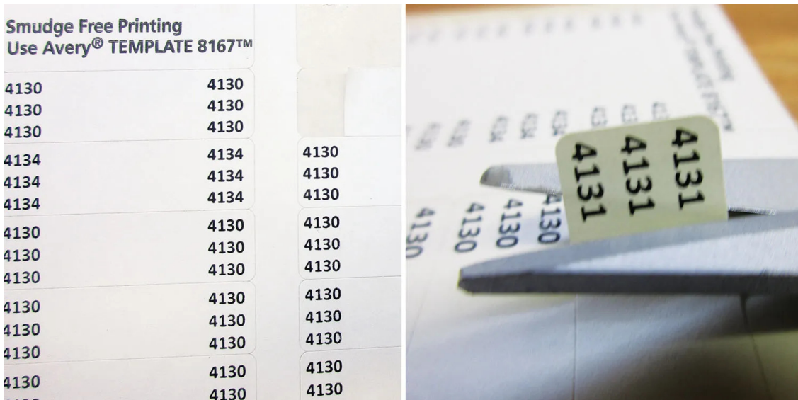
Avery return address labels for wires beginning with wire #4130 (left). Please use a laser printer. Cutting off the useable half of the label for one end of the wire (right).
