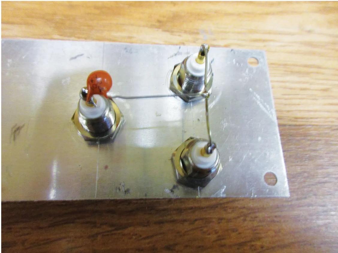
The glideslope coupler for a VOR/LOC antenna.
