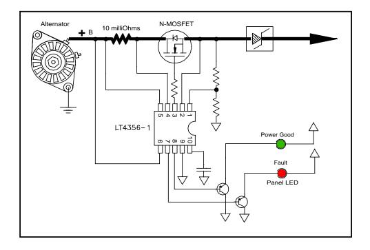
So what happens? Normally the alternator current is carried by the N-MOSFET. Assume the current is 50A, and the Rds(on) is 0.012 ohms. The dissipation would be only 30W. This is easy to handle with a reasonable heat sink.
