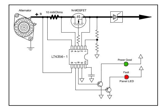
So what happens? Normally the alternator current is carried by the N-MOSFET. Assume the current is 50A, and the Rds(on) is 0.012 ohms. The dissipation would be only 30W. This is easy to handle with a medium-sized heat sink.
