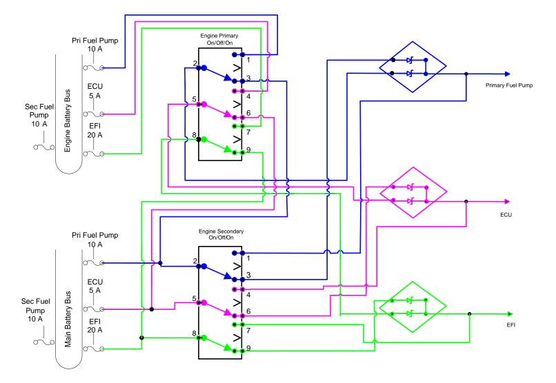
Notes: This is an adaptation of Z19 drawing for Eggenfellner Subaru H6. Use 3P3T (On-Off-On) Switches (2 needed) NKK P/N S33F (20A @ 30V DC) or P/N S833 (30A @ 30V DC). Use Perihelion Design Power-Deuce-Schottky Auto-Power Diode Assembly (3 required).
