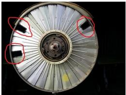
6. **Remove Outer Ring Braces.** You will have to take the outer ring braces loose that attach the ring to the nine cylinders. Do not lose those spacers at the base of those L brackets that mounts them to the stud on the cylinders. They are impossible to find replacements.
