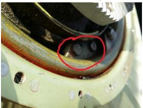
4. **Loosen Nose Case Bolts.** Look around the base of louvers there are ? 11 mm bolts that bolt the ring to the nose case. Slowly loosen them all together so you are going loosen one a little, move to the next one, then the next one until you have all the walked around the ring. That is because over the top of the bolts is a slot in the perpendicular ring that prevents the bolts from backing completely out if they loosened in flight.
