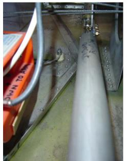
I then took a 3x5 card and taped it on the control foot. I took a fine line ink pin and marked the holes already there for the cable clevis forks had bolted on. Because the push rod Male Rod End Bearing bolts required more distance apart then the existing holes I had to make and add a bracket..
