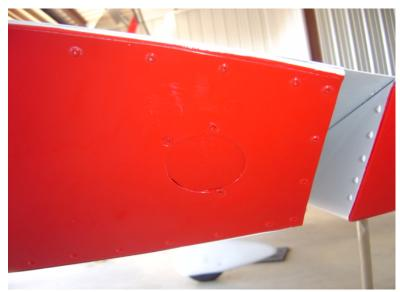
rear edge. I cut a 1 1/2 inch hole with the door knob hole saw or you could use a fly cutter.
