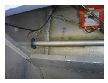
Once I attached the inboard bolts through the Eye Bearing bolts into the foot, I placed a brace support under each aileron to flush it with the flap.
