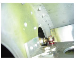
I removed the marked rods from the wings, trimed to the correct length, installed the second pair of insert plugs, drilled and riveted as before.
