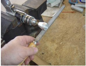
I ordered four rod ends from Van's (VA-111 Threaded Rod Ends & M 361 M Rod End Bearing) and machined them down with a file until they fit tight in the tube ends. Your source for the tube ends may vary or you might get Dave Nixon to make you some as he did for his plane.
