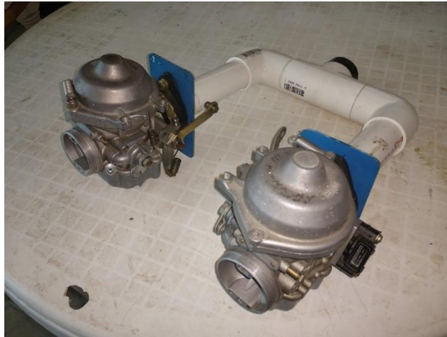
Vacuum cleaner setup to check carb pistons.
