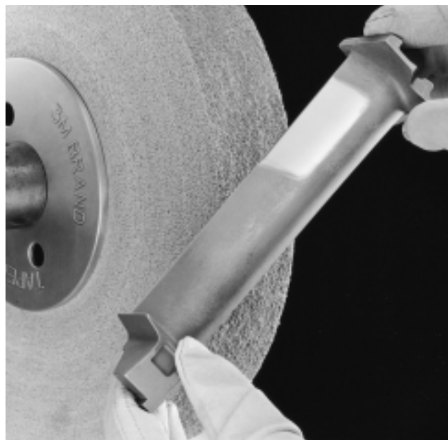
Jet blade deburring – Scotch-Brite EXL deburring and finishing wheel radiuses leading and trailing edge without chamfering or undercutting.
