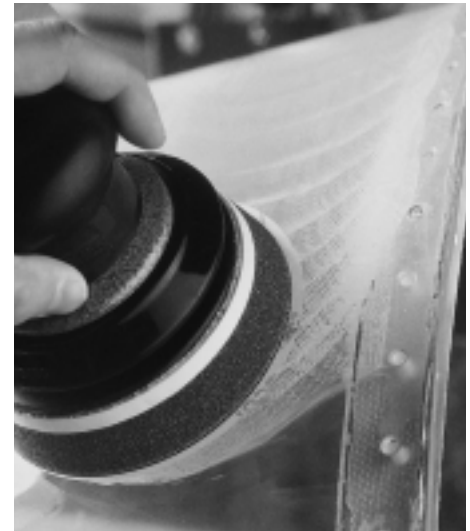
Jet canopy maintenance – 3M™ Imperial™ microfinishing film removes pitting, scratching, and crazing.
