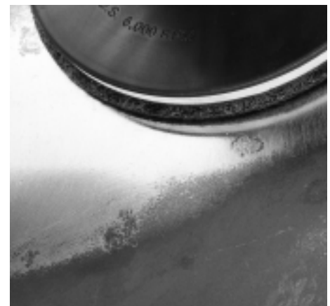
Coatings (left) and corrosion removal (right) – Scotch-Brite surface conditioning disc removes coatings and corrosion. Controlled abrasive action helps prevent undercutting or gouging. Fresh abrasive is continually exposed to the work surface for consistent, uniform results.
