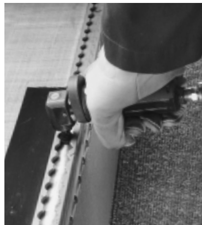
Seat Track Cleaning – Scotch-Brite Roloc surface conditioning discs fit within the seat track to efficiently clean and remove corrosion.
