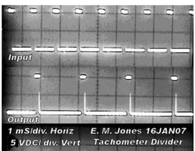
achometer sending units provide some number-of-pulses per revolution. This can be a problem if you have more than one sender or receiver or mismatched units. So if you have 3 pulses per revolution and need 1.5, or have two but need one, you need a divider.
