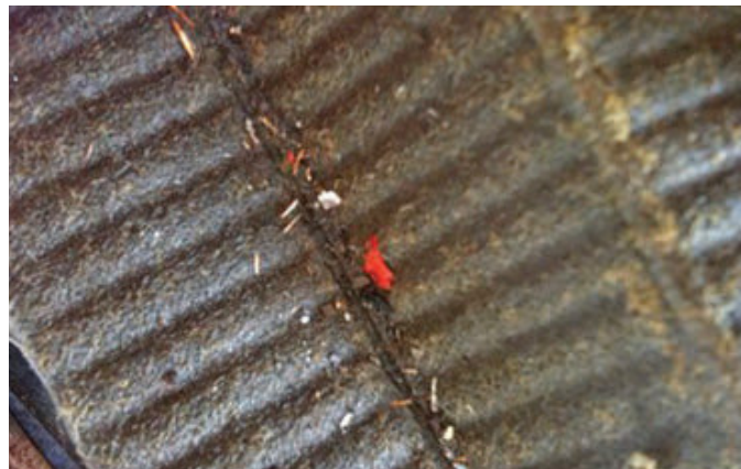
Figure 2. This oil filter media contains hundreds of ferrous metal whiskers, most likely from cam and/or lifter spalling. The engine will likely need a teardown.
