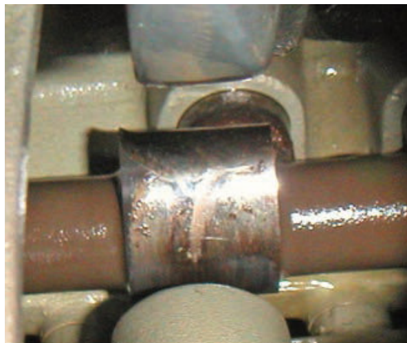
Figure 3. Badly damaged cam lobe found during cylinder removal. It's time!
