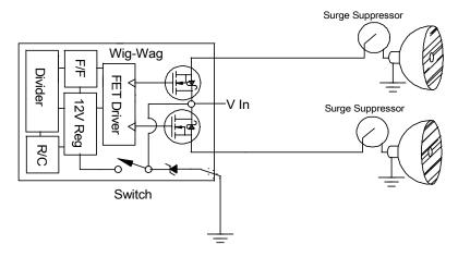
As the wattage of the lamps increase, more care has to be taken to keep the current through the Mosfets inside the Wig-Wag within operational limits.
