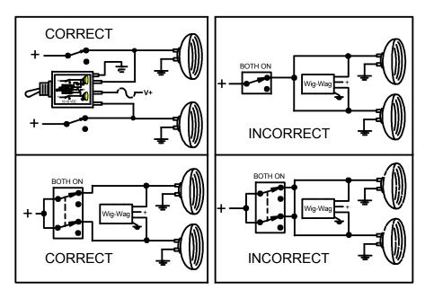
Note: Occasionally someone calls because their installation doesn't work, usually because the installer neglected to make sure that each lamp CAN operate independently so that it can be wig-wagged. Often a landing and taxi light are wired to operate together. This can be done several ways. So be sure that each lamp can operate independent of the other.
