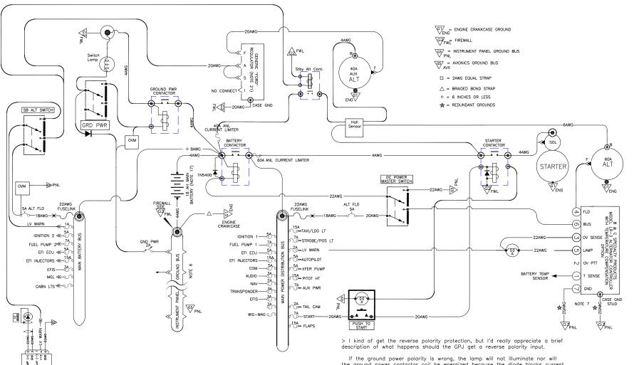
If the ground power polarity is wrong, the lamp will not illuminate nor will the ground power contactor coil be energized because the diode blocks current in the reverse direction.
