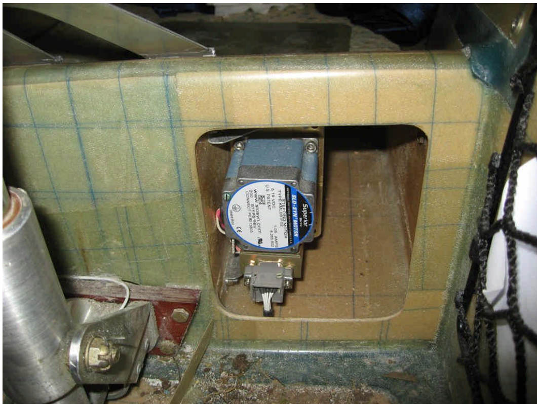
Picture 2 Example TruTrak installation
