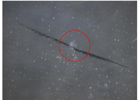
Figure 6: Magnified view showing sand on the inner fracture surface
