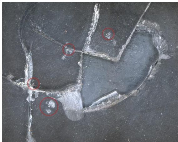
Figure 4: Close-up of the canopy puncture showing several impact marks (circled)
