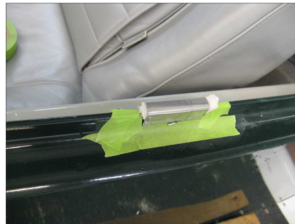
FIGURE 4: EPOXY/FLOC OOZE-OUT AROUND SAFETY LATCH WEAR PLATE
