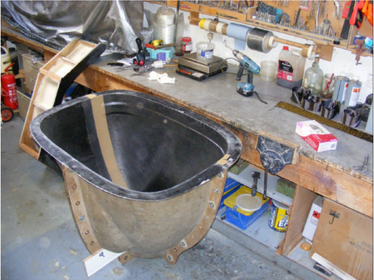
Top and bottom cured, now the location flange gets laminated
