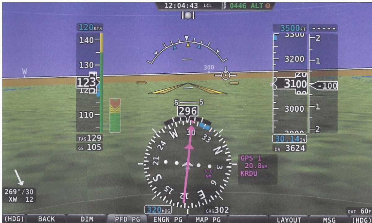
Fig.3 The latest Dynon Skyview EFIS with AOA display. In earlier versions the AOA was a bit more prominent
