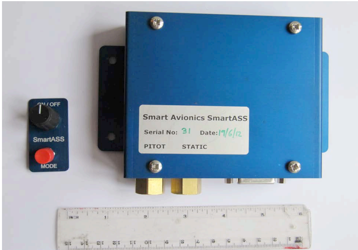
Fig 3. The control panel and box. A prewired connecting system is included in the kit.
