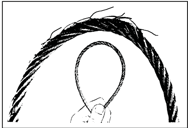
FIGURE 7-16. Cable inspection technique.
