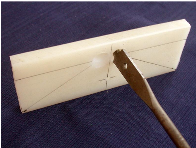
Figure 5 – Countersinking the two antenna terminal holes with a 1/2" wood bit.
