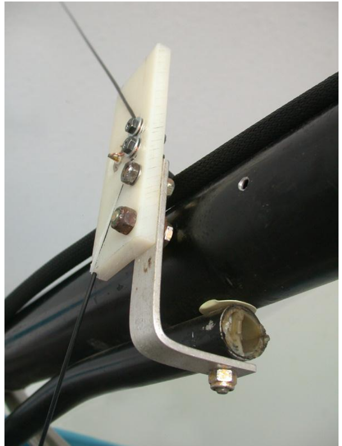
Figure 14 – Antenna mounting example using an L-bracket. Anything similar will work as well.
