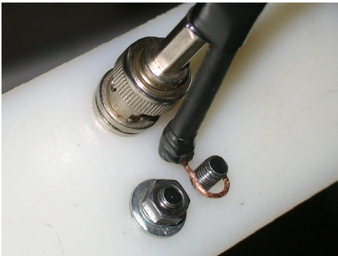
Figure 13 – Connecting a wire loop "pigtail" on one end of the Pawsey Stub to the center conductor antenna terminal. Shown before securing with washer and nut.
