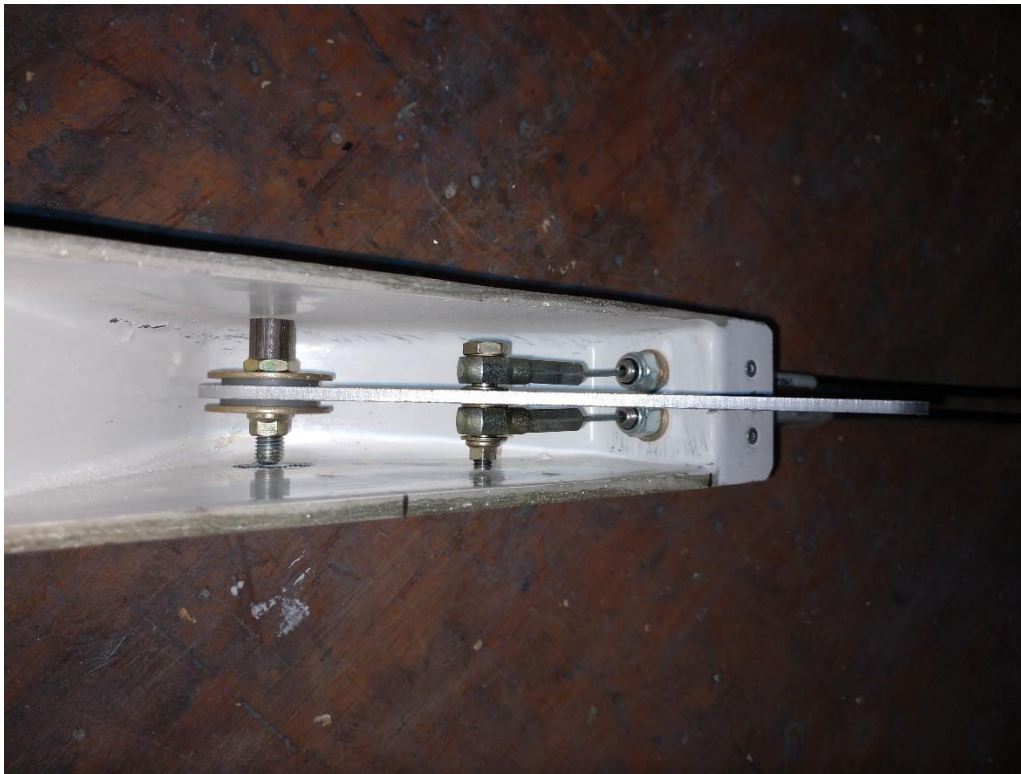
Photo of a typically built throttle box.
