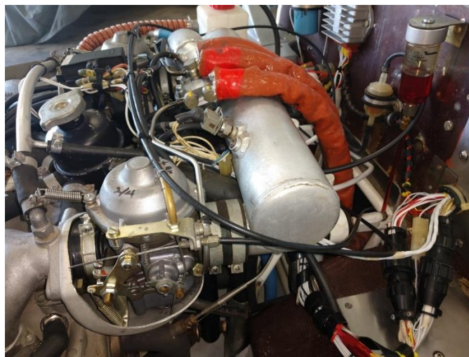
Photo of 12AY showing choke cable runs.
