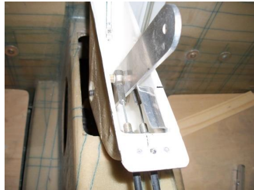
Basic Throttle Idle and 100% Detent Stop
