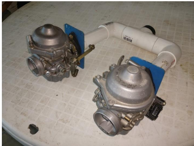
Vacuum cleaner setup to check carb pistons.
