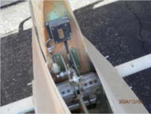
Trim & Stabilator Assemblies
