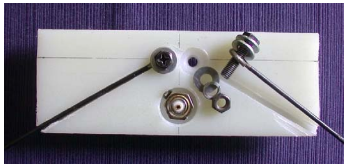
Figure 8 – Mounting the antenna elements and BNC connector.
